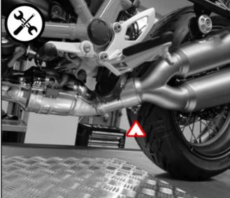
Remove the stock muffler.
