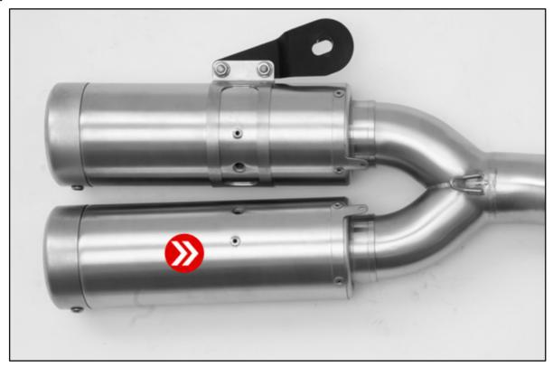
Mount the supplied exhaust bracket with the supplied hex socket screws to connect the two mufflers. Hook the two springs.
